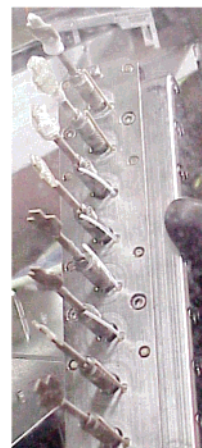
Figure 7. Photograph of the stirrers from a parallel reactor which shows the difference in solubility of different polymers produced as the percentage branching increases, as the loading of the oligomerization catalyst ( 3 ) is increased from zero (top reactor) to 400 nmol (bottom reactor). The photograph was taken after the reactors were cooled and vented.
